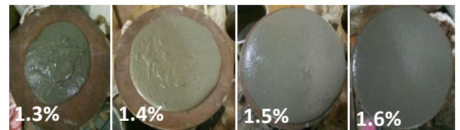
Figure 2. Influence of Super Plasticizer on the mortar mixture: (a) 1.3%, (b) 1.4%, (c) 1.5% and (d). 1.6%.
